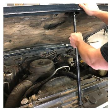
This installation refers to the driver side. All steps are to be repeated on the passenger side in kind. You will want to begin by propping the hood up in a position to where you can easily access the factory hinge assemblies.
