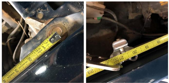
Measuring from the center of the rear fender bolt to the center of the ball stud, you will need to clamp the lower strut mount into position. Using some tape between the clamp and aluminum will help protect the aluminum from being damaged. To achieve different open heights, you can use the following measurements: For Maximum Height (closest to stock): 20.5 Inches. For Minimum Height (lowest opening to still have access to engine bay): 22 inches Recommended height: 20.75 Inches
