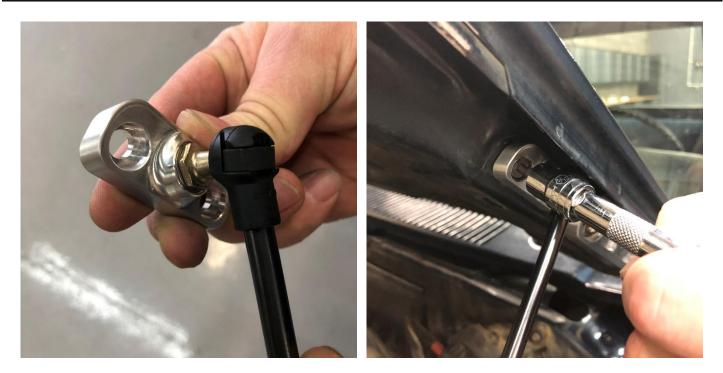
The strut will need to be attached to the upper mount prior to fastening it to the hood. Using the 5/16 screws provided, fasten the upper mount to the hood as shown.
