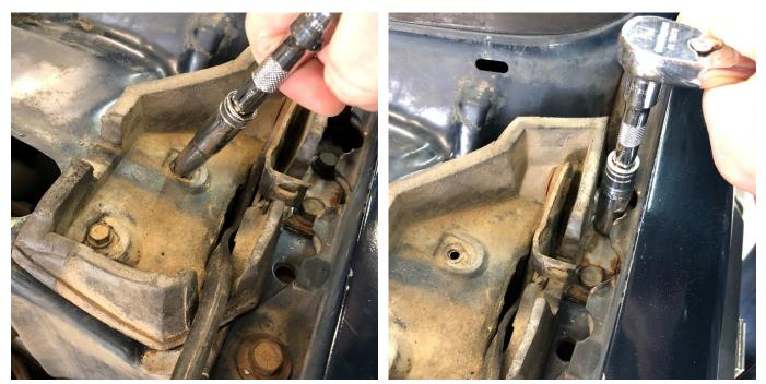
Remove the 4 bolts attaching the hinge to the cowl. These will no longer be used.
