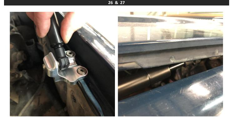
Once the upper mount is attached to the hood, you can then attach the strut to the lower mount. Remove the hood prop and slowly lower the hood. Keep an eye on the strut to make sure it compresses properly and does not run out of travel. Also check to ensure the strut isn't rubbing painted surfaces of the hood or fender. If it does, the strut mounting studs can be shimmed out by using 5/16 washers.
