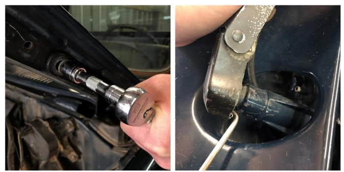
Remove the hood from the hinges. Be careful not to drop the hood damaging the cowl panel or fenders. Remove the wiper arms. The retainer, shown in step 5, will be pulled away from the stud allowing the arms to come off. You will need to apply upwards and downwards pressure to adjust the angle of the assembly to allow it to come off straight. Do not force it off at angle, it can damage the stud causing you to not be able to properly reinstall the wipers.
