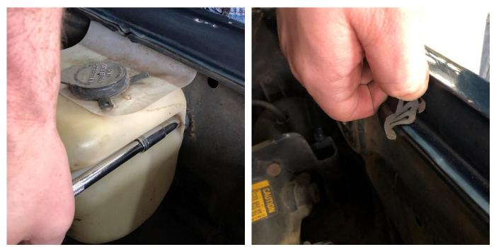
If the truck has the factory washer reservoir installed, you will need to remove it at this time. Remove the rear rubber bump stops from the fender.
