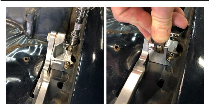
Using the 3/8 bolts and washers provided, attach the new hinge assembly to the cowl. Do not tighten them all the way down at this time. Allow a little wiggle room for the hinge to be adjusted from side to side. Install the original clips used to attach the cowl panel onto the hinge.
