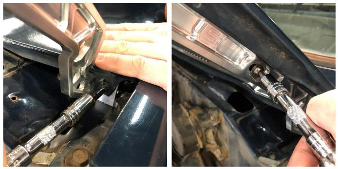
We recommend removing the hood from the truck before reinstalling the cowl panel. Reinstall the cowl panel with the original hardware and then reinstall the wiper arms. Once the cowl panel is on, you can now install the hood for the final time. Make the necessary adjustments to align the hood from front to rear and tighten the arms into position. Once the hood is aligned and secure, prop the hood into the open position.
