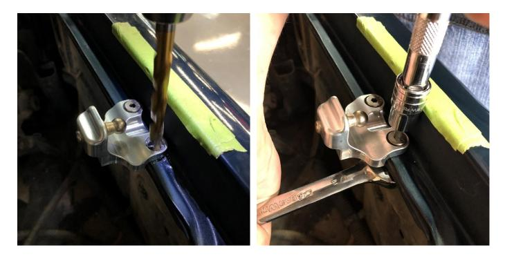
Once one side is tightened, remove the clamp and repeat drilling/fastening on the other side.
