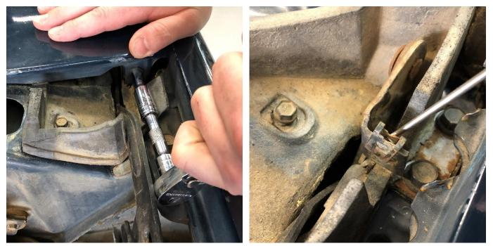
There are 4 screws along the front edge that will allow you to remove the cowl panel. Then remove the 2 outer clips from the hinge. **Do not discard the clips. They will be used on the new hinge.**
