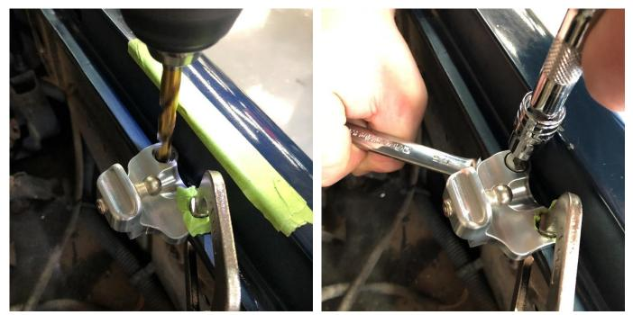
Once you have the mount clamped into the correct position, use a 5/16 bit to drill the holes for the fasteners. Use a 5/16 screws and nyloc nut to fasten the mount to the fender after the first hole is drilled.
